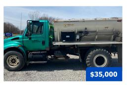
**2003 International 4400 Spreader,** DT466 210 hp diesel engine, Eaton 10-speed trans., air ride seat, 11 ft New Leader L2000G4 spreader, Ag Leader Insight controller, light bar, roll tarp, front 385/65R22 (30% remains), and rear 48x31.00-2tires (50% remains). Motor had a major overhaul 60,000 miles ago, new radiator, and clutch.
