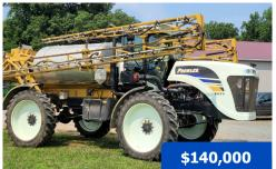
**2012 GVM E275 Prowler**, 642 hrs., Cummins QSB 6.7L, 6-cylinder, Tier 3, 275 hp diesel engine, all-wheel drive mechanical drivetrain, ZF WG210 powershift, 6 speed trans., 1600-gallon SS tank, 70/90 ft booms, 20 in. nozzle spacing, 5-way nozzle bodies with SS boom lines, poly chemical eductor, Raven Viper Pro, Phoenix 200 receiver, Raven SmarTrax Autosteer, Goodyear 380/90R46 tires (50% remains).
