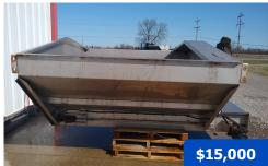
**2017 Double Duty 7' Insert,** 7 ft multi-product insert, fits in 13 ft spreader body, 304 SS. All electrical and hydraulic connections included.
