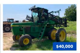
**2005 John Deere 6700**, 3,986 hours, 4-cyl PowerTech 2240 turbocharged 106 hp diesel engine, hydrostatic trans., 2-forward gears, 420 gal. poly tank, 60 ft booms, 15 in. nozzle spacing, EZ Guide 250, A/C, AM/FM radio, crop shields, fenders, front tires 12.4-38 (45% remains), rear 13.50-16.1SL (50% remains).
